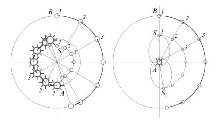
Figure 11. Motion of the satellite at the interior collinear libration point.
